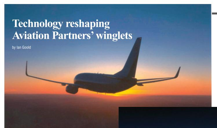
Pushing the technology envelope as far as physics will allow. Aviation Partners' winglets research has succeeded in minimizing drag and improving performance. The firm has introduced winglets for the Raytheon Hawker 800 series (below) and Boeing Business Jet (left), and is said to be on the verge of bringing the technology to other models as well.
