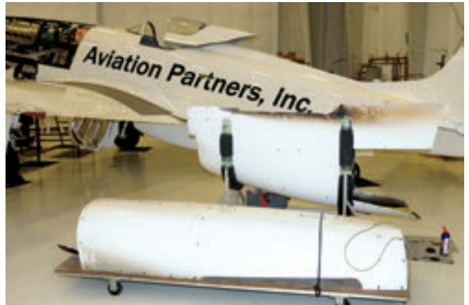
The innovative two-piece composite cowl in just one of the many design features on Voodoo that aid in the aircraft’s quest for speed. “It certainly makes it easier to remove and put back on compared to the standard cowl,” comments Bernie Vasquez. (MOL)
